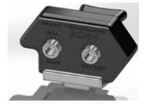
Both the gain and offset are set at average values from the factory. You can adjust the values to customize your Breath Controller.
